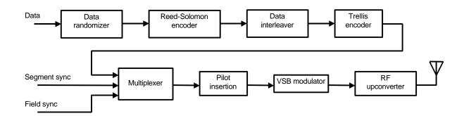
The baseband data signal is filtered with a complex filter to produce in-phase and quadrature components for orthogonal modulation. These two signals are converted to analog signals and then used to quadrature-modulate the IF carrier creating a vestigial sideband IF signal by sideband cancellation.
