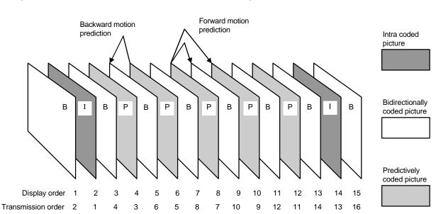
Figure 5. Example of a coded video sequence using I-frames and P-frames and B-frames.
