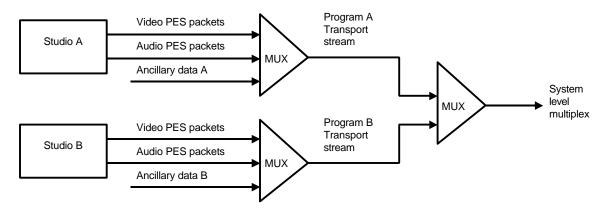
Figure 10. System level multiplex.
